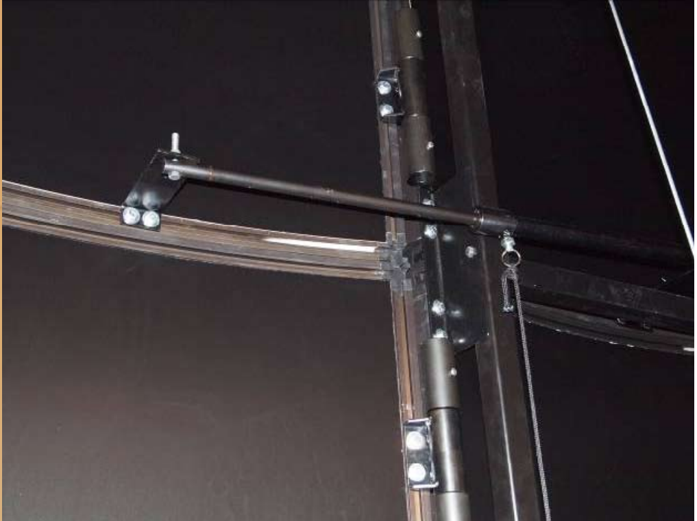
3.5 A telescoping wing lock device locks tower wings in performance or storage positions.
